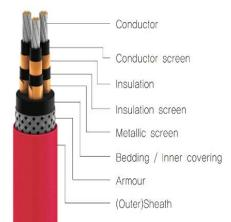
Braid armour: Tinned copper wire braid (O), Galvanized steel wire braid (C) Outer sheath: Halogen free thermoset compound SHF2 or halogen-free MUD resistant thermoset compound SHF MUD complying with IEC 60092-360(359) and / or NEK
