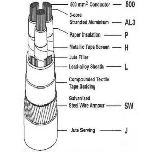
11kV 500 AL3 P H L SW J 11 kV phaseto-phase 500mm2 3-core strandedaluminium conductors, paperins ulated s creened, lead alloy s heathed s ing lew irearmoured jute s heathed(cable code 351 – s ee Annexure D). SW- GalvanisedSteel Wire Armour.
